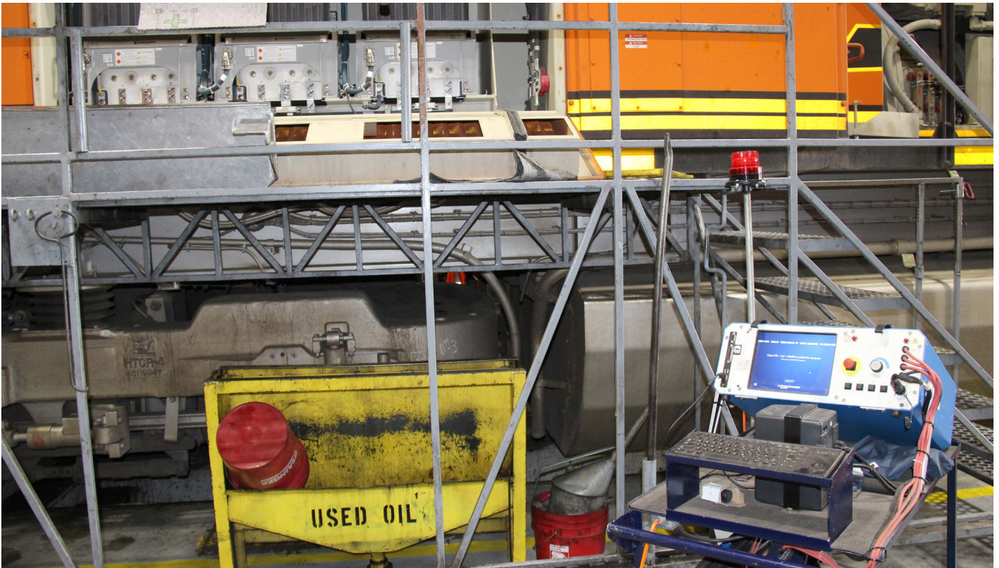
The Baker AWA-IV is used for testing AC traction motors in locomotives in maintenance and repair depots at leading railway companies throughout the world.
